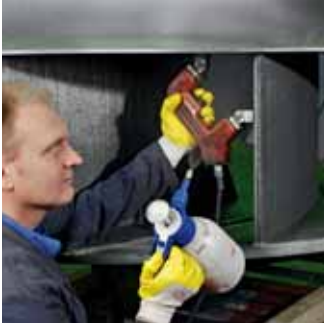
Surface crack check (MP) on the weld after the repair has been carried out
