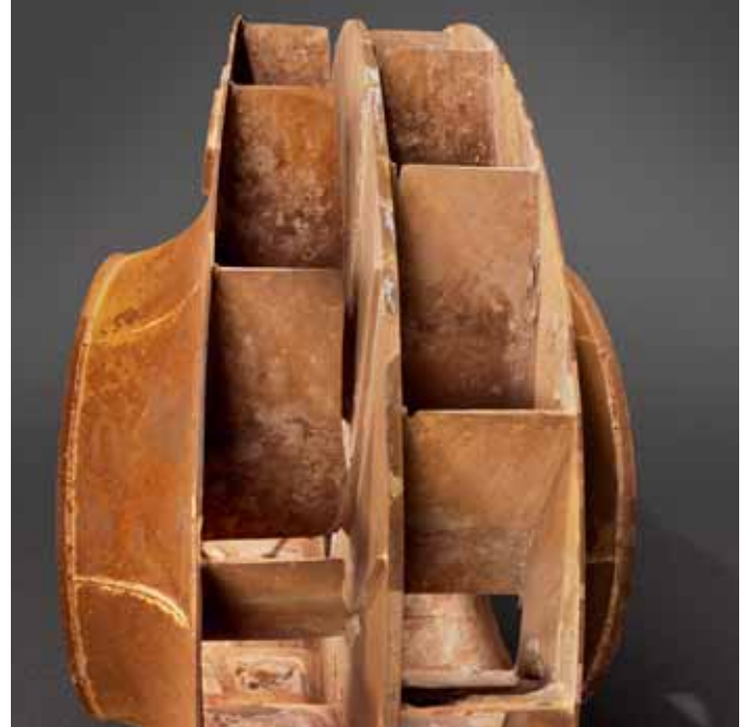
Damaged impeller without wear protection
