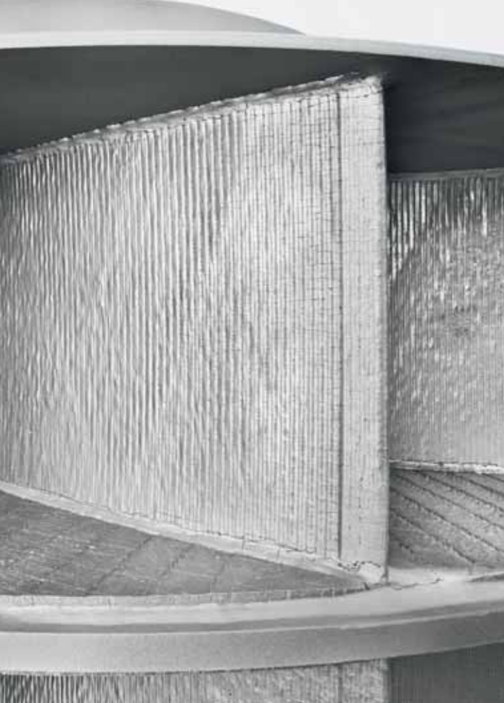
Special wear protection on the critical areas of the impeller
