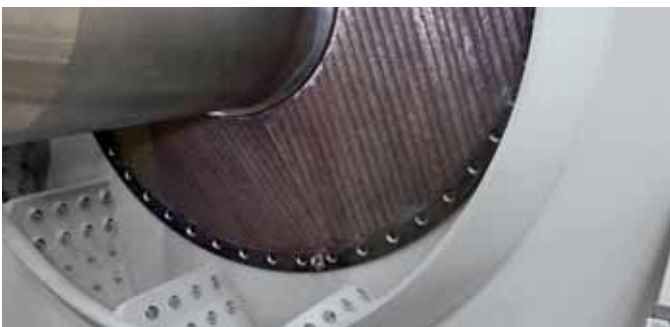
Wear-resistant cover for flanged connection
