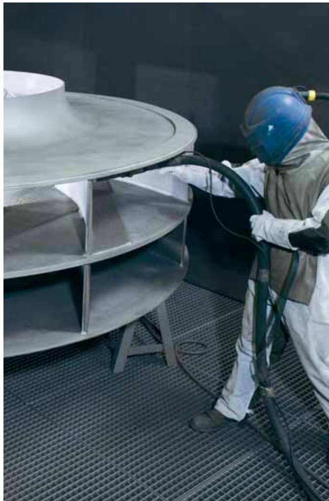
Cleaning a double-inlet impeller before damage analysis
