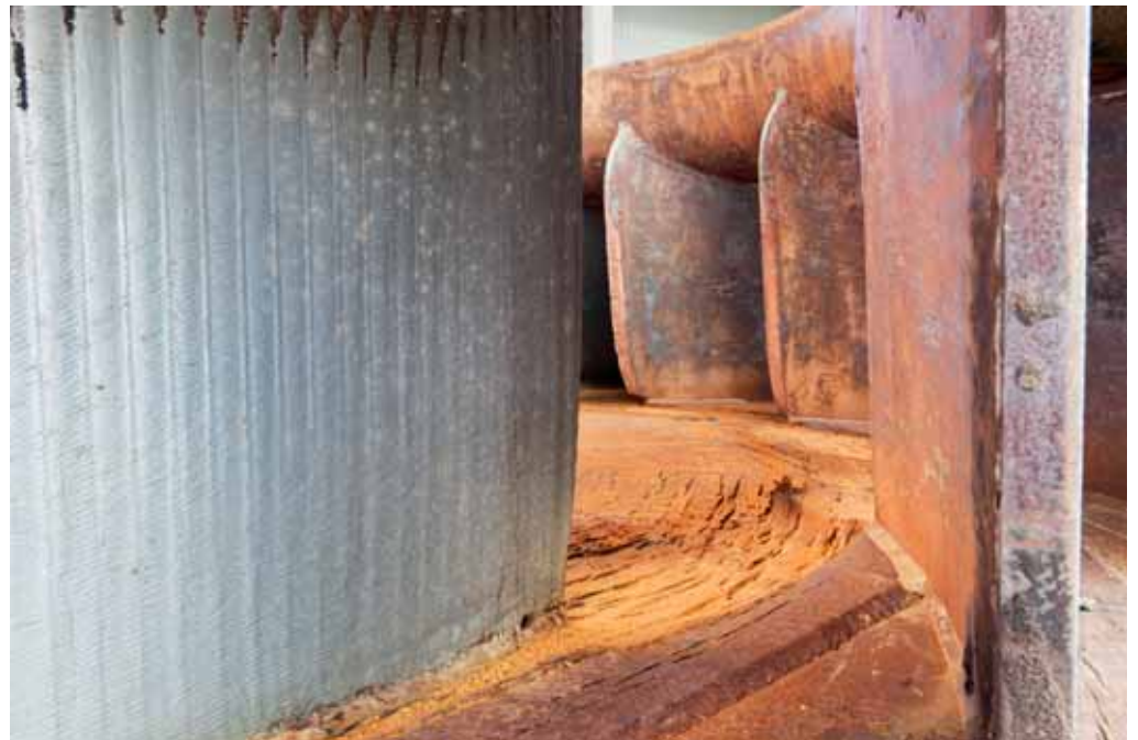
Impeller with wear on the centreplate
