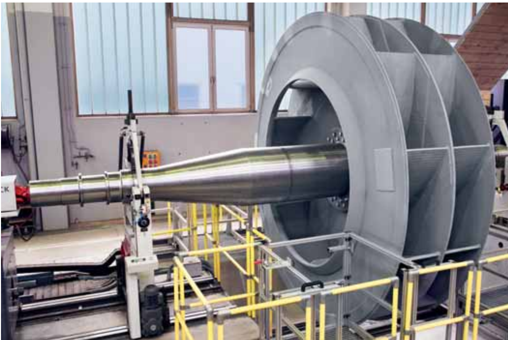
Balancing a double-inlet rotor
