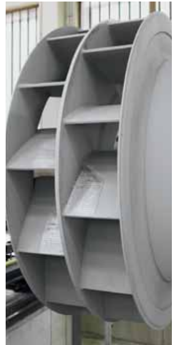
Specific protection against wear in areas of the impeller blade
