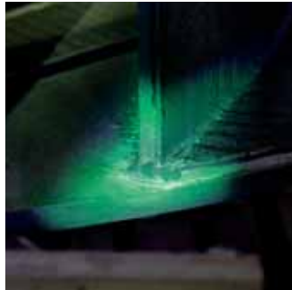
Surface crack check (MP) on the weld after the repair has been carried out
